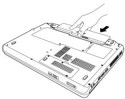
(Sample Illustration) Inserting the battery
